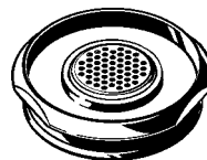
The Dosing Capsule inserted into the Filling Chamber Reducer
