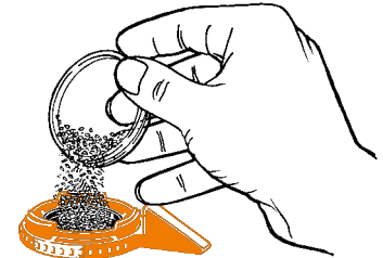
Always fill the Filling Chamber completely up to the upper edge
